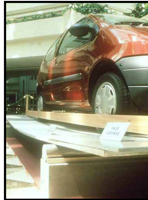
2,000 lb car on a 1 ¼ -inch sheet of Ductal®
