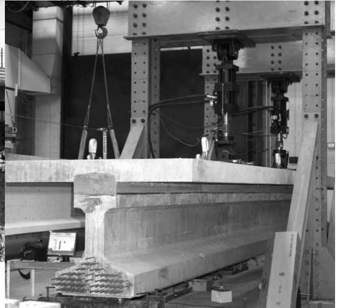
Right: UHPC composite connection test specimens are subjected to cyclic loading.
