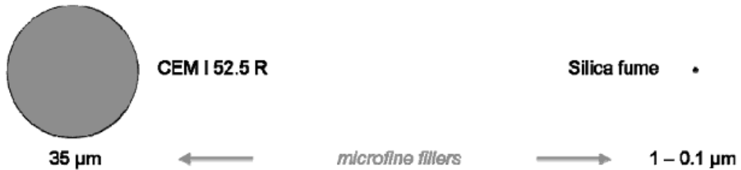
Figure 10 To fill the voids between the cement particles, a larger amount of silica fume is needed [34]
