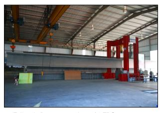
Full scale flexure strength test for TBG1325-29.5m.
