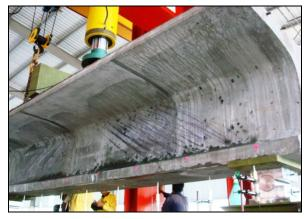
Full scale shear strength test for TBG875-8m
