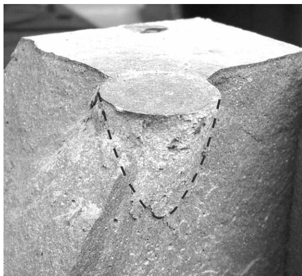
Figure 6: Concrete wedge under the loading area
