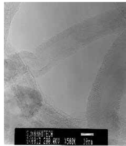
Figure 2: TEM-image of MWNTs, SUN Nanotech Co Ltd. [8]
