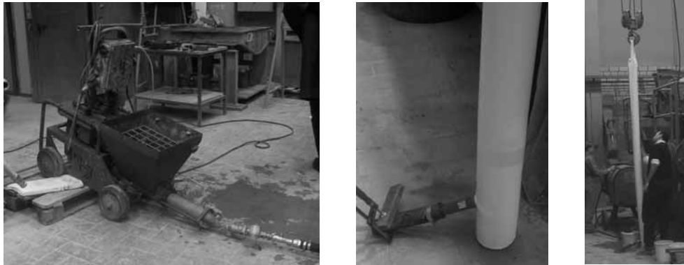
Figure 7: Spiral pump type PFT N 2V and filled 3m membrane tube \varnothing 12cm
