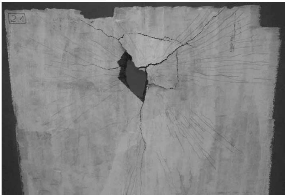
Figure 11: crack pattern in plate 2.1 (200 * 200 * 3 cm) edge load
