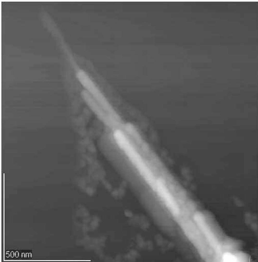
Figure 3: Bundle of CNTs imaged by AFM on HOPG
