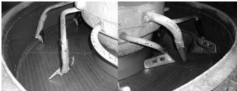
Figure 2: Ring mixer (mix volume 1000 l)
