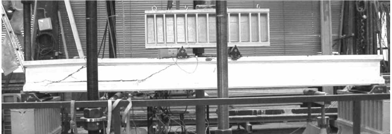
Figure 10: Test specimen in a state of failure
