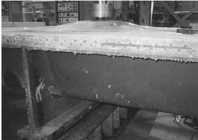
Fig. 8. Fatigue tests on a bridge deck with high performance fibre concrete [8]
