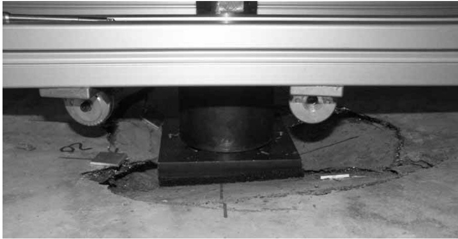
Figure 14: crack pattern in the plate 2.1 (200 * 200 * 3 cm) on the top side
