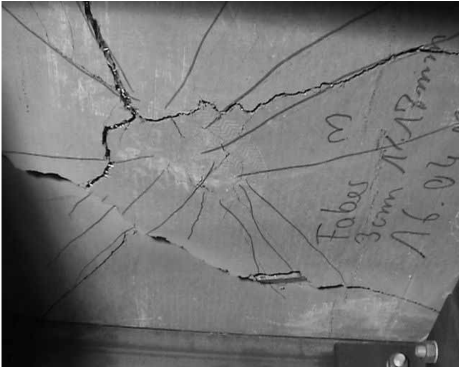
Figure 12: crack pattern in plate 2 (100 * 100 * 3 cm) centre load
