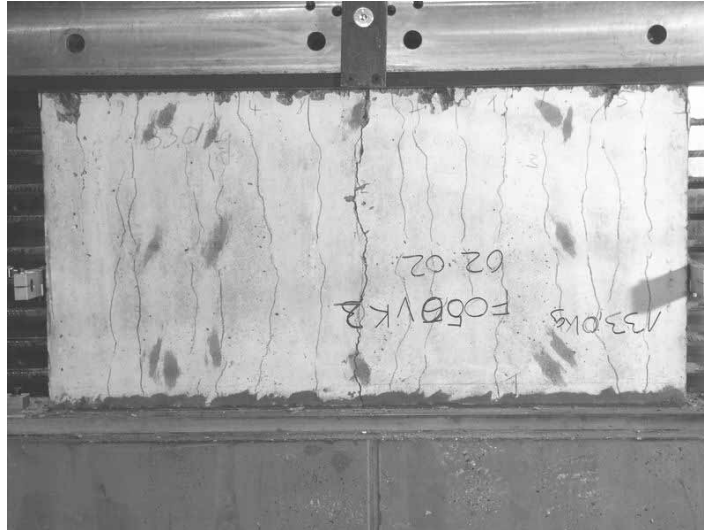
Figure 8: Opening of only one crack in the middle of the panel at a strain of 5.5 ‰
