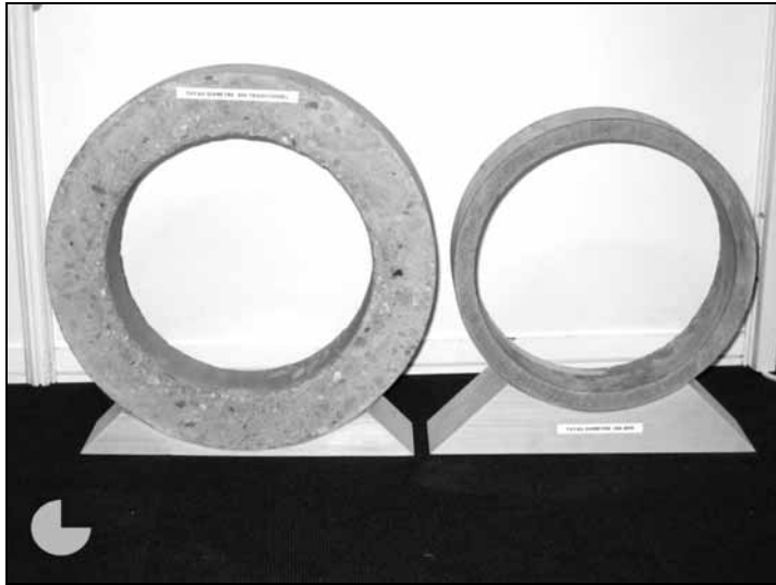
Figure 9: Use of ultra high performance concretes in sewage pipes
