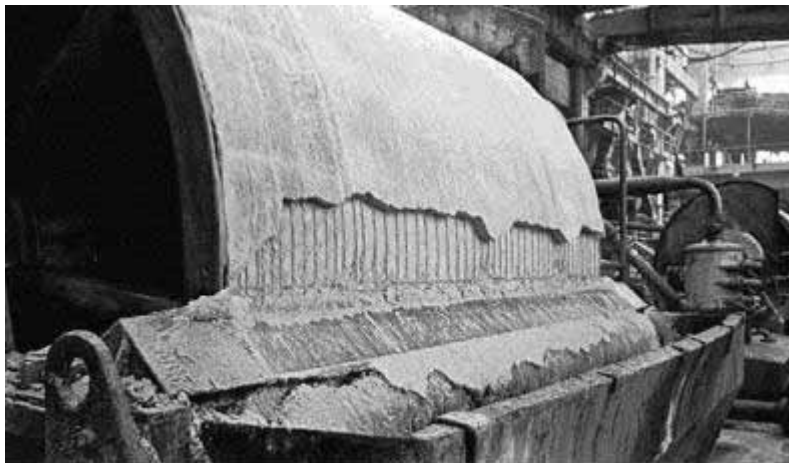
Figure 14: Filter Vacuum Rotary Drum
